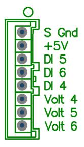
An ignition expansion is provided allowing you to convert to a Direct Spark ignition system. Alternatively these outputs can be used to drive auxiliary devices. The following pinout describes the available connections.
